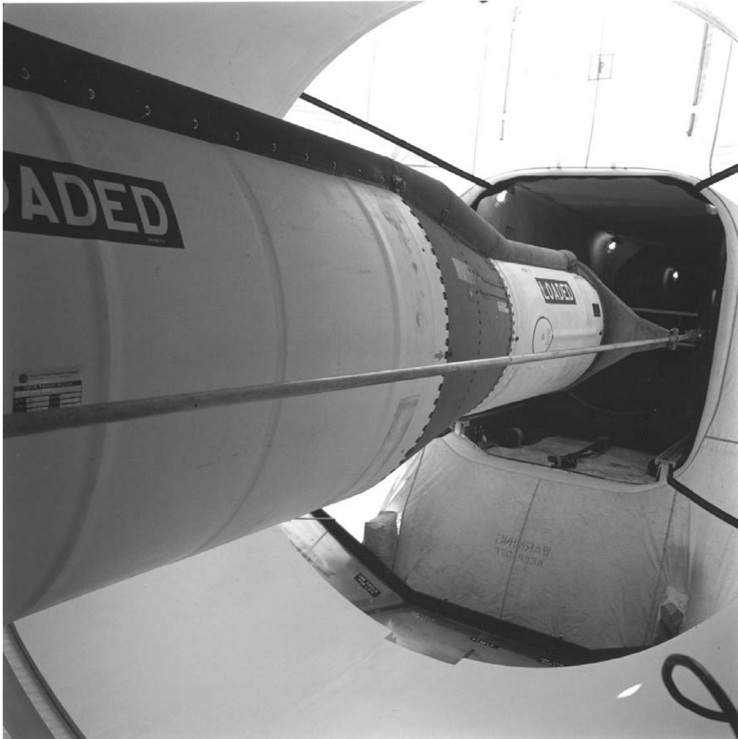
Plate 52. A Delta Flight missile being emplaced in the Transporter Erector ( Library of Congress, Prints and Photographs Division, Historic American Engineering Record, Reproduction Number HAER SD- 50- C-18 )
