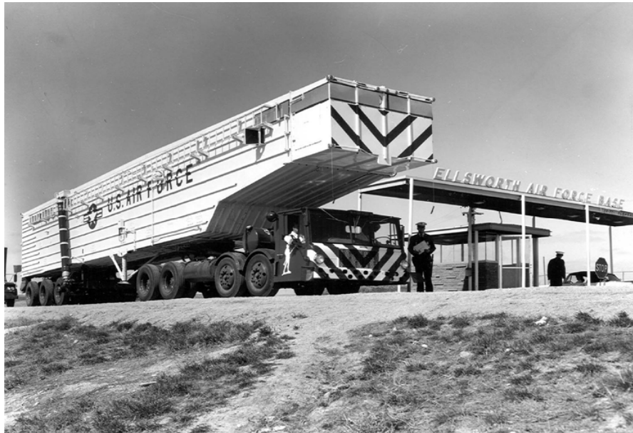
Plate 19. Transporter Erector at Ellsworth Air Force Base ( "Site Activation Chronology, Minuteman Project, Ellsworth Air Force Base, South Dakota, July 1963- October 1963," K243.012- 40, in USAF Collection, AFHRA )
