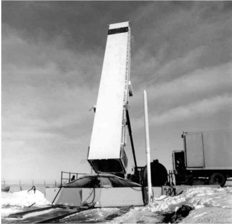
Plate 77. Transporter Erector positioned to remove missile, Delta Flight ( Library of Congress, Prints & Photographs Division, HAER SD- 50- C- 7 )
