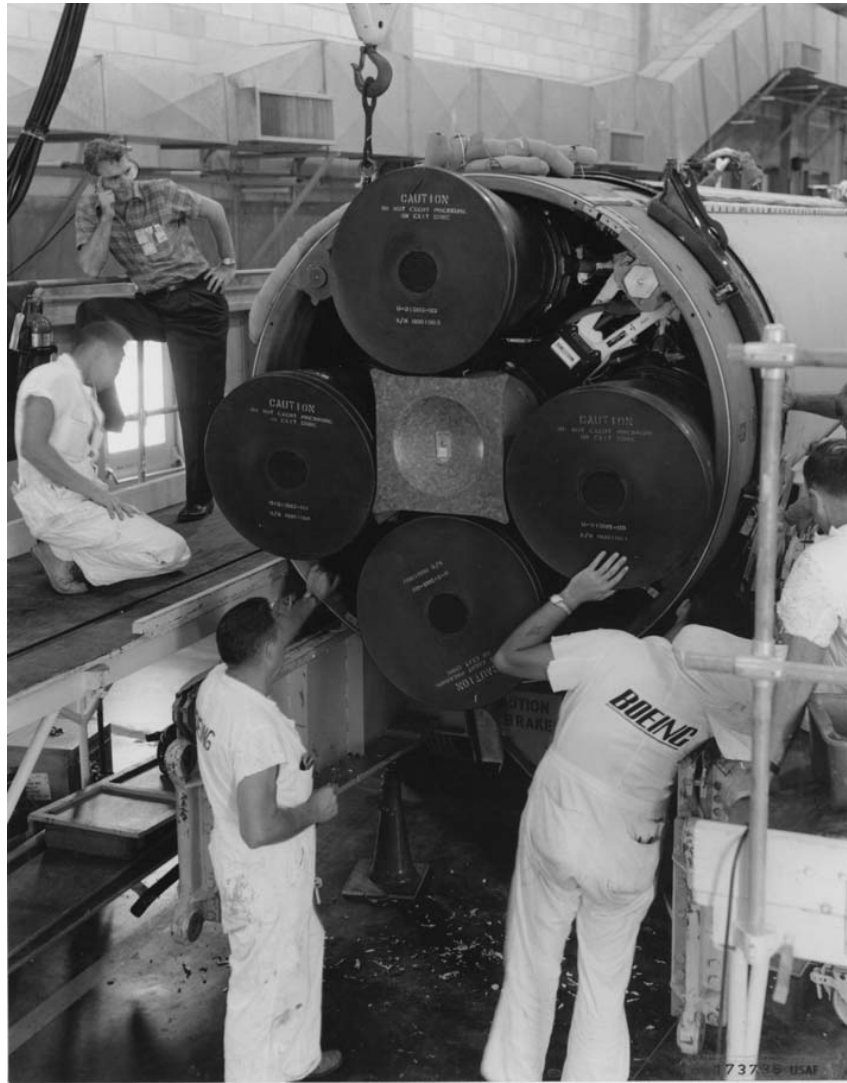
Plate 35. A Boeing crew assembles a first-stage Minuteman engine at the Air Force Missile Test Center, Cape Canaveral, Florida, 14 June 1963 (Photograph No. B-08-018-1, "Guided Missiles - Boeing "Minuteman," U.S. Air Force Photo, Record Group 342, National Archives, Washington, D.C.)
