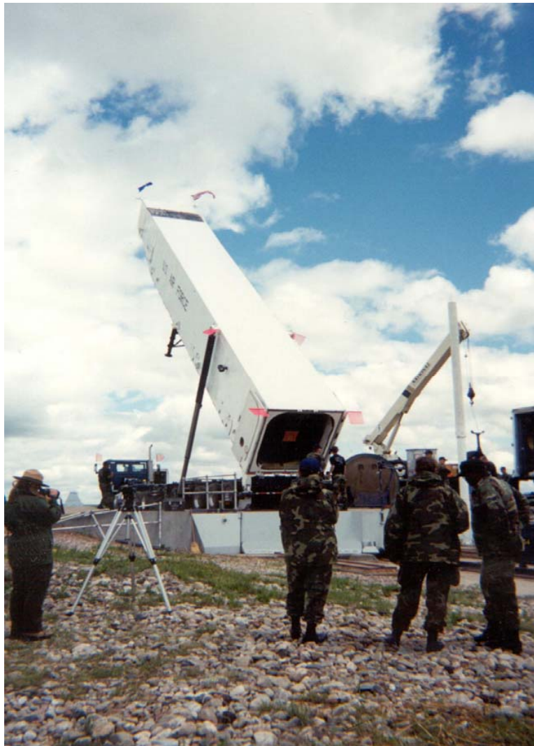
Plate 83. Transporter Erector ready to emplace the training missile at Delta-09 (Courtesy of the 28 th Civil Engineer Squadron, Ellsworth Air Force Base)
