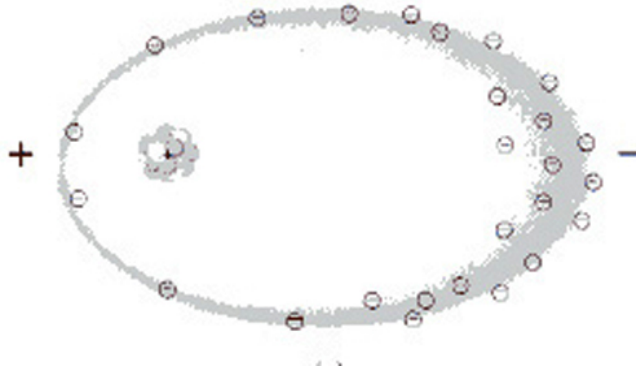
Figure 62. In a constant external propelling field, the electronic orbits of atoms are distorted, creating a negative space charge where the orbits are most distant from the nucleus.
