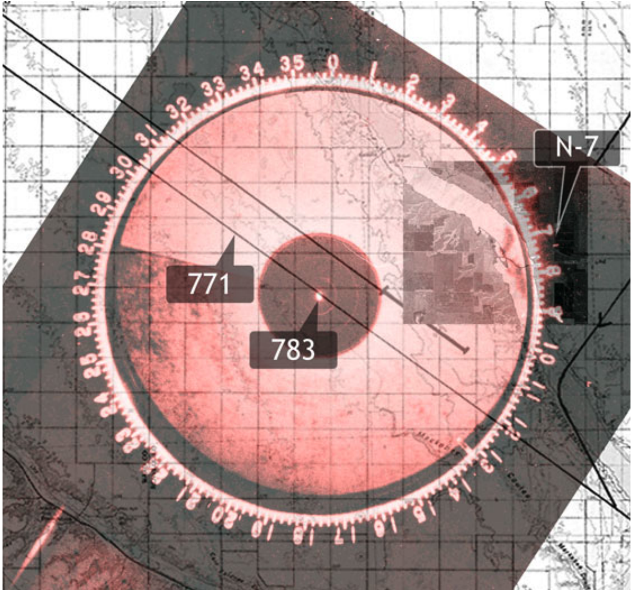
Figure 39. The extreme positions of the B-52 during the radarscope photos. Photo 783 has been rotated to the true course of the B-52 at 122 degrees on approach to the runway, and scaled to match the underlying USGS map with Werlich Overlay, and satellite image of Lake Darling. The B-52 covered 2.65 nm over the course of the photos, and was 18.8 nm from the TACAN at the most probable altitude of 8865 feet MSL during 783. (USGS map with Werlich Overlay available from: http://www.minotb52ufo.com/mapsnew/usgs_poher.php ).
