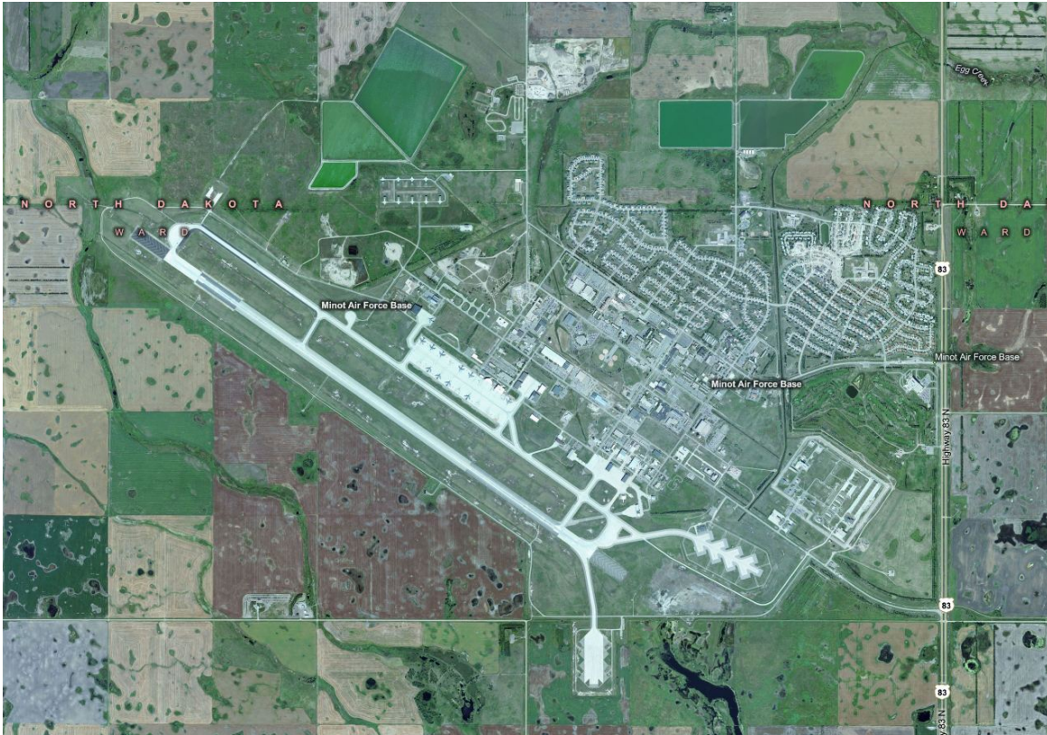
Figure 7. Satellite image of Minot Air Force Base. The runway length is 13,197 feet (2.5 miles, or 4.02 kilometers). 3
